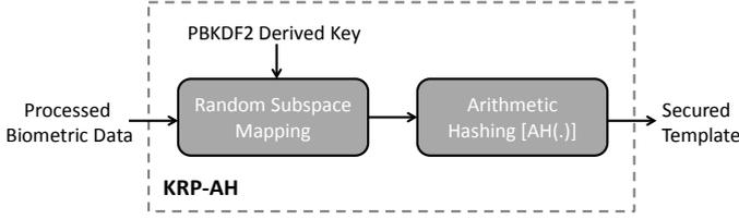
Figure 1: KRP-AH Scheme for Secure Template Generation
