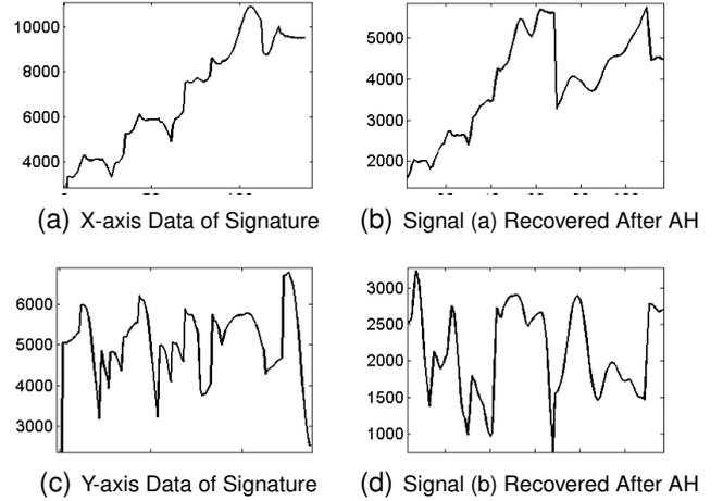
Figure 3: Arithmetic Hashing Hinders the Recovery of Original Signal: The left column shows original signals and the right column shows signals recovered by interpolation (up-sampling) followed by integration of the output from AH function. Handwritten Signature for demonstration is taken from sample data in SVC dataset.
