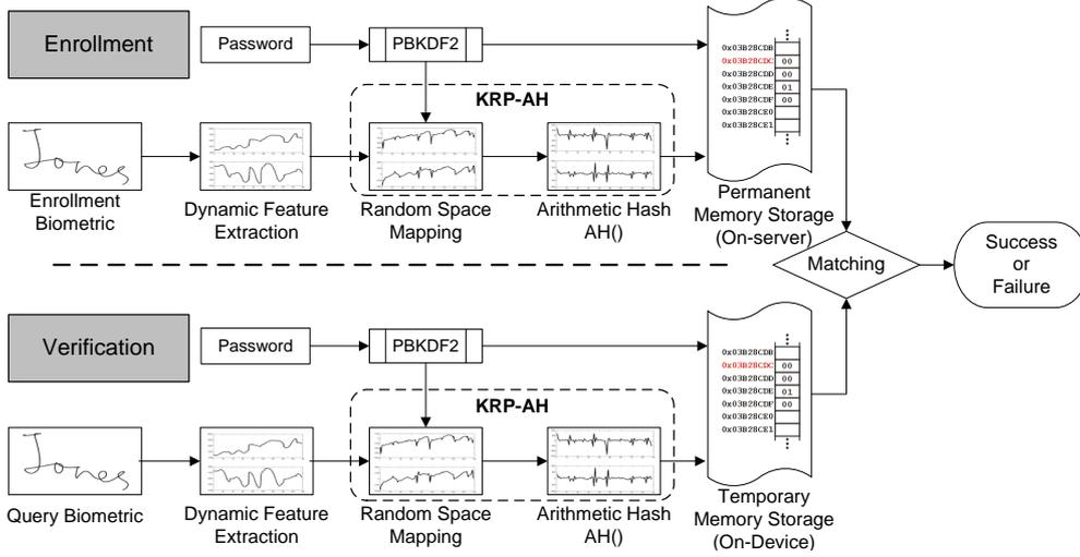
Figure 2: Complete architecture of bi-stage two-factor user authentication framework using KRP-AH scheme
